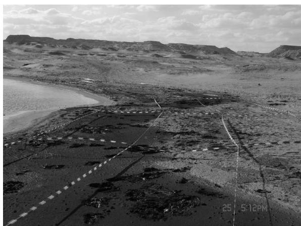
Fig. 2. Contaminated soil by crude oil at the bank of produced water disposing pit at oilfield.
