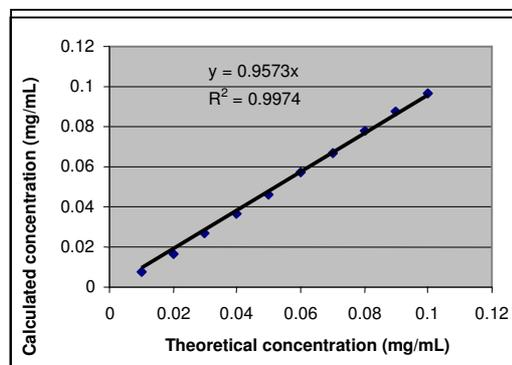
**Fig. 1** - Linearity results using the optimized UV spectrometric method
