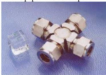
**Fig. 1.** Cross Flow Micro Heat Exchanger realized at Forschungszentrum Karlsruhe
