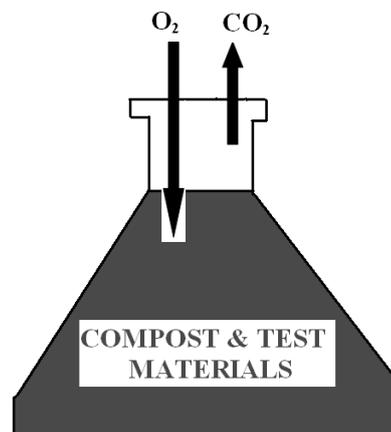
**Fig.1.** Experimental installation for the mineralization of materials in soil column
