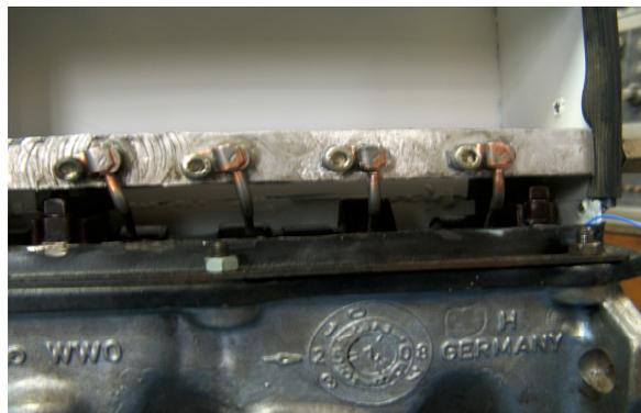
**Fig.6.** Rail for additional lubrication
