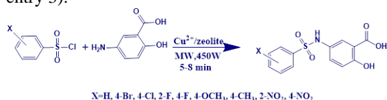
Scheme 1. Synthesis of substituted mesalazines.
