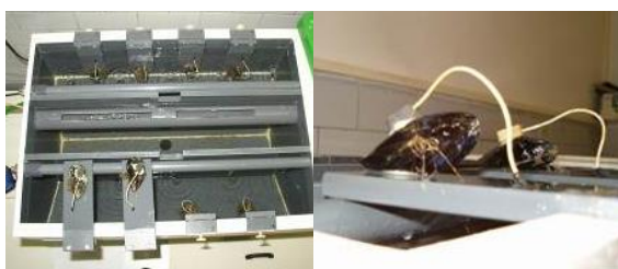
Figure 2. Placement of M. galloprovincialis into Mosselmonitor®.
