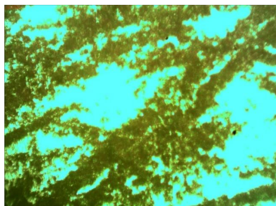
Figure 5. Micrograph of steel surface after exposure for 24 h in 1.0 M HCl.
