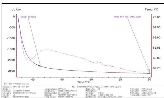
**Figure 10.** Creep curve of unreinforced wLDPE at 70 °C
