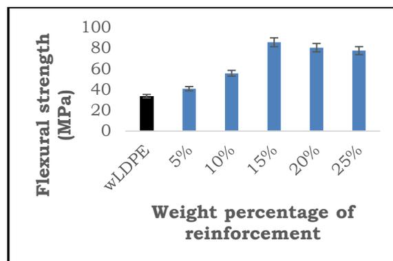
**Figure 3.** Effect of plantain peel powder on the flexural strength of waste LDPE composites
