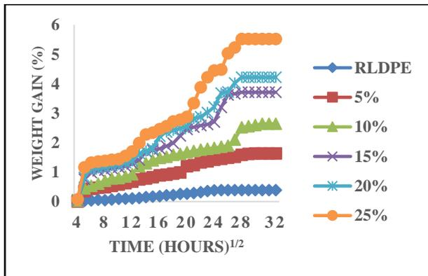
Figure 5. Water absorption curves of the composites immersed at RT for 30 days.
