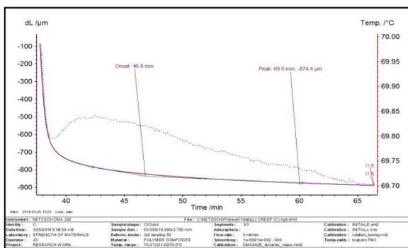
**Figure 9.** Creep curve of 15 % plantain peel reinforced waste LDPE composites at 70 °C
