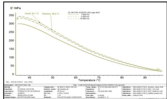
Figure 7. Storage modulus curve of 15% wt plantain peel powder reinforced waste LDPE composite at 1, 5 and 10 Hz.
