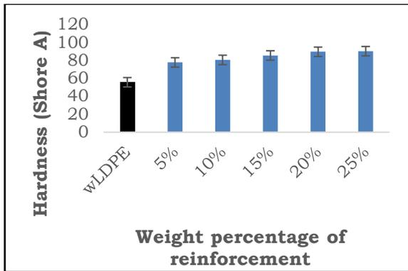
Figure 4. Effect of plantain peel powder on the hardness value of waste LDPE composites
