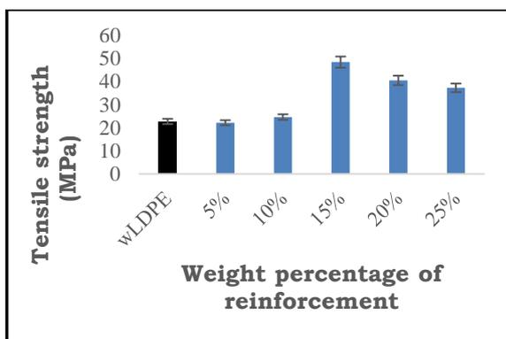
**Figure 1.** Effect of plantain peel powder on the tensile strength of waste LDPE composites
