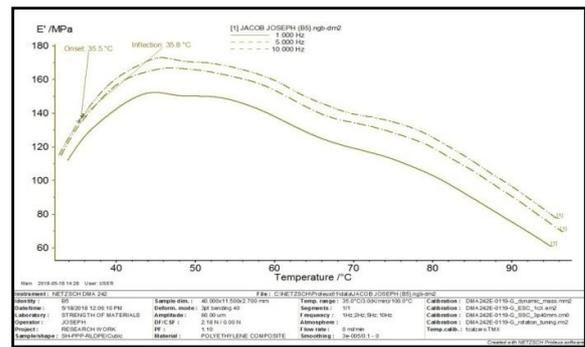
Figure 6. Storage modulus curve of waste LDPE at 1, 5 and 10 Hz.
