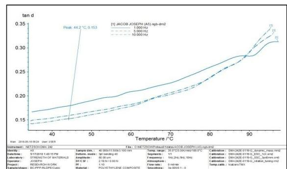
Figure 8. Damping curve for 15 % wt plantain peel powder reinforced waste LDPE composite at 1, 5 and 10 Hz
