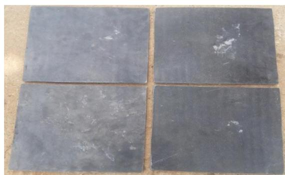
**Plate III.** Some of the developed potential composite wall tiles.
