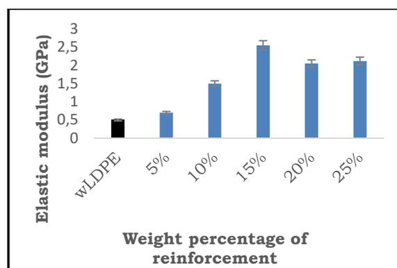
**Figure 2.** Effect of plantain peel powder on the elastic modulus of waste LDPE composites
